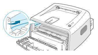
**5** Grasp the handle and insert the cartridge in the printer until it snaps into place.
